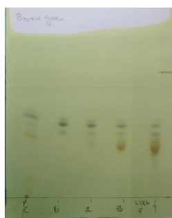
Figure 22. - Picture of a TLC plate stained with Bromocresol green.
