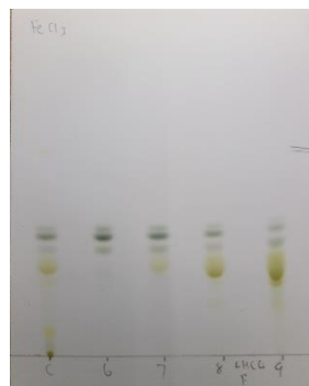
Figure 20. – Picture of a TLC plate stained with Iron (III) Chloride.
