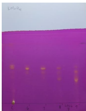
Figure 19. – Picture of a TLC plate stained with potassium permanganate.
