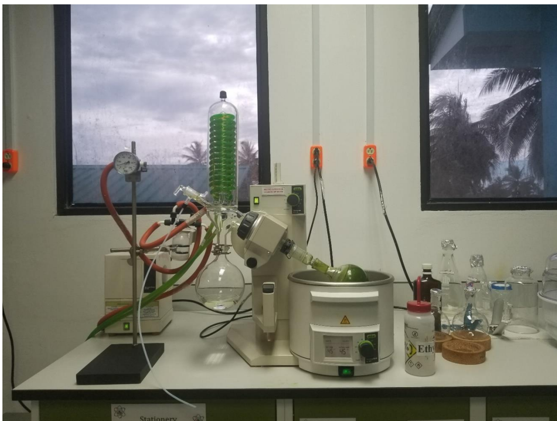
Figure 40.– Picture of the Rotary Evaporation of the solvent being done with a Buchi R 210.
