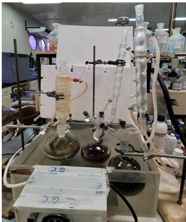
Figure 42.– Picture of the reflux setup – water bath, flasks, sample, and condensers (cold).
